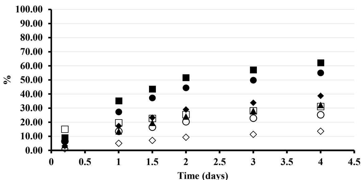
**Figure S1.** Release of tannic acid by the time from a G/TA<sub>x</sub> matrix made from 1mg gelatin and expressed as a percentage from the initial TA content. (◇) G/TA<sub>15</sub> (○) G/TA<sub>30</sub> (□) G/TA<sub>50</sub> (▲) G/TA<sub>70</sub> (◆) G/TA<sub>100</sub> (●) G/TA<sub>150</sub> (■) G/TA<sub>200</sub>.
