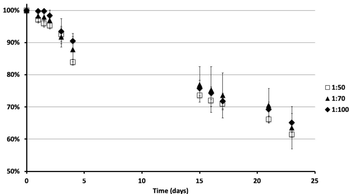
**Figure S2.** Time evolution of the area of G/TA<sub>x</sub> matrixes incubated in citrate/phosphate buffer pH = 7 at room temperature. One could note the shrinking over the time period. There is no difference in the three different G/TA molecular ratios tested.
